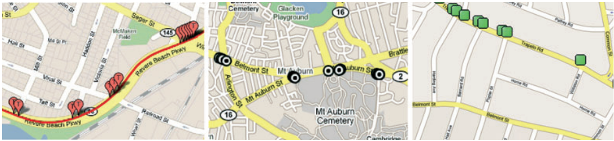
Figure 4. A computer program has been developed to identify, from GPS recordings, segments where the vehicle crosses junctions. The class of roads or junctions can be specified. For example, we can select only junctions with limited access roads (pins on the left figure), major road intersections (circle markers on the middle figure), or minor streets (square markers on the right figure).
